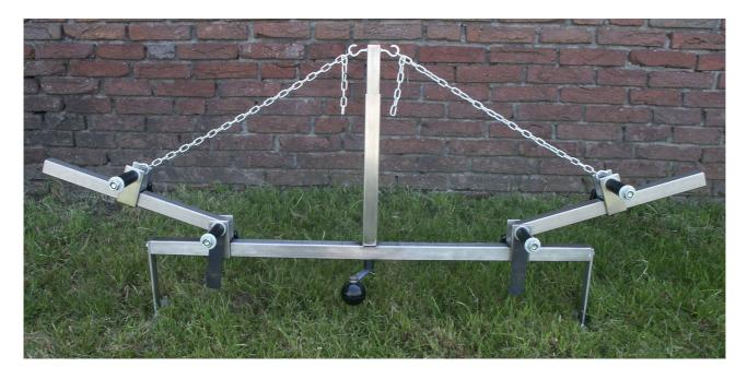
This is it: a bowpress that will fit any bow. It's cheap to build, very rugged, and doesn't need a lot of expensive machining: in fact, the one pictured above, built in stainless steel costed me about \$100.
