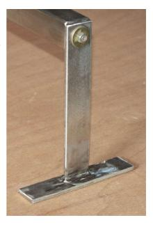
If you're a little bit of a DIY guy you can do the rest yourself with simple tools: File, hacksaw, fine sandpaper and a knife to cut the rubber tubing. Get rid of any sharp edges, sand it down, paint it if you want to or sand/polish it when it's stainless steel.
