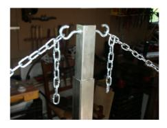
5: Put the 2 pieces of chain on both sides: The excess chain hanging down in the middle makes it easy to see if you're working symmetrically.
